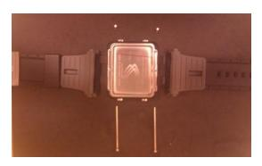
**5.** Replace the battery and mount back all the screws, the long screw can be a bit hard to press into the hole
